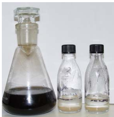
Waste water samples On the left: before treatment On the right: after treatment
