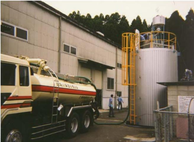
The purpose of this Biogas plant is the use as test and demonstration plant in mobile applications for treatment of odd quantities of organically high loaded sewage water and sludge.
